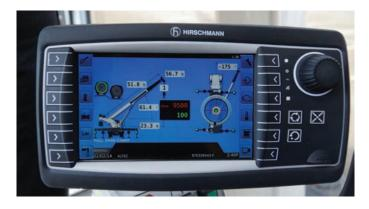
The convenient LMAP menu navigation with an intuitive user interface displays load on hook, rated capacity percentage, boom length and angle, load radius, and operator-defined protection with audible alarms. While the intuitive display and user interface are unique to Altec, the system's hardware consists of common "off-the-shelf" components that were critically selected for their performance and serviceability.
